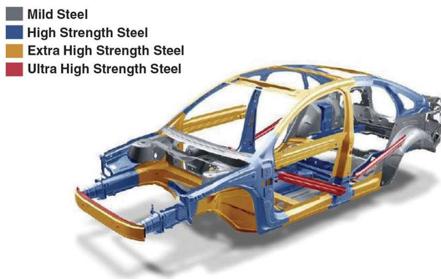
Figure 2: Types of steels used for each body part (50)
