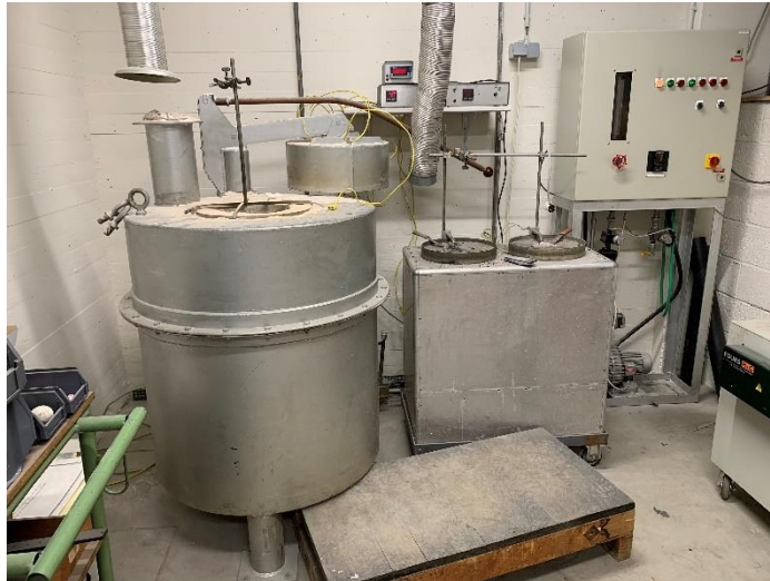
Figure 25: Fluidized bed furnace (left) and lead bath furnace (right)
