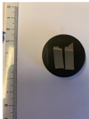
Figure 43: Macroscopic fracture surface for 750-30 - A (left) and 750-30 - B (right)
