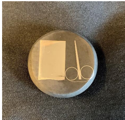
Figure 21: Polished and etched sample for microstructural analysis with the flat part (left) being a sample through the length and the thin (right) a sample along the thickness.
