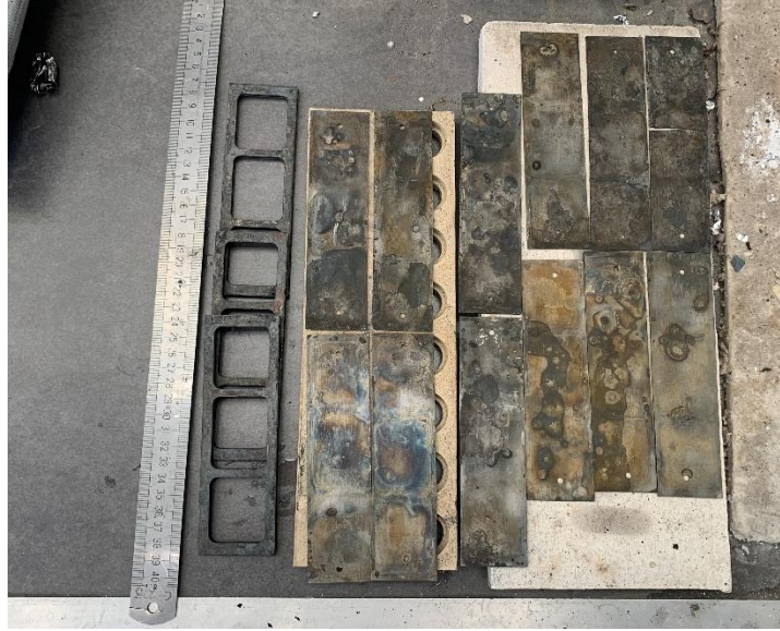
Figure 19: Specimens casings on the left part of image and austenized specimens on the right part
