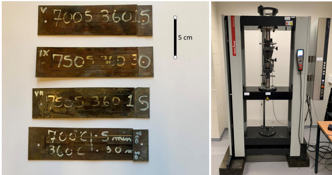
Figure 27: Machined tensile specimens (left) and tensile tester (right)
